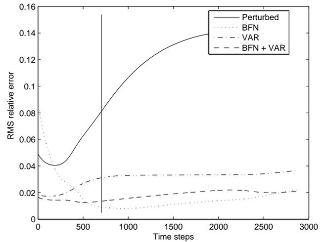
**Fig. 9.** Evolution in time of the RMS difference between the reference trajectory and the perturbed trajectory derived from the noisy observations of the system at time  $t=0$  (full line), and between the reference trajectory and the identified trajectories for the BFN (dotted line), VAR (dash-dotted line) and BFN-preprocessed VAR (dashed line) algorithms, in the case of noisy observations (with a 5% RMS error).
