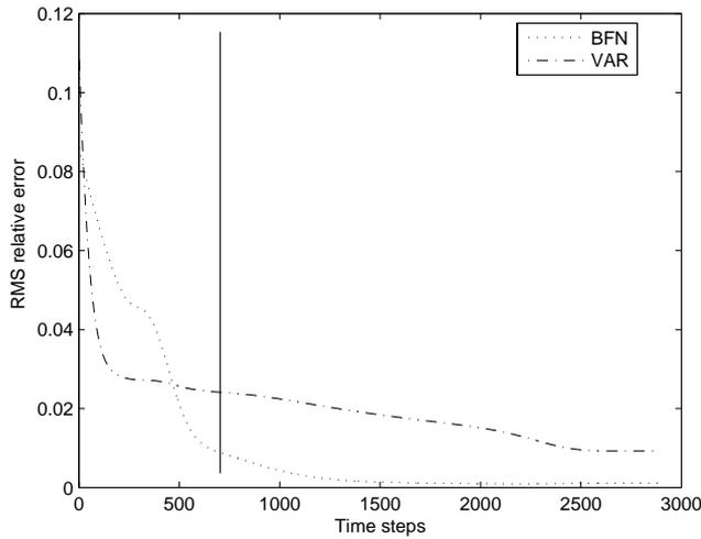
**Fig. 8.** Evolution in time of the RMS difference between the reference trajectory and the identified trajectories for the BFN (dotted line) and VAR (dash-dotted line) algorithms, in the case of perfect observations.
