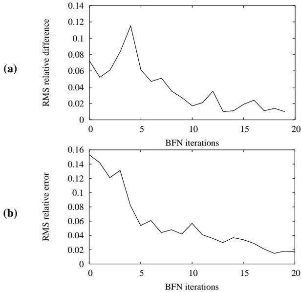
**Fig. 17.** RMS relative difference between two consecutive BFN iterates (a) and between the BFN iterates and the exact solution (b) versus the number of BFN iterations in the case of an imperfect model.
