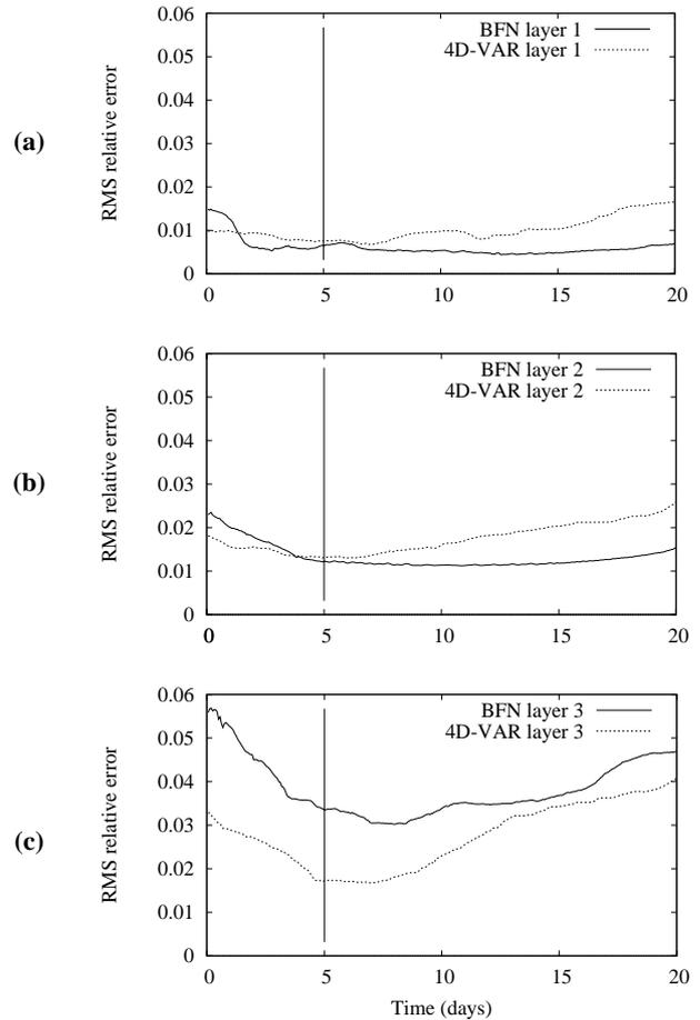
**Fig. 16.** Evolution in time of the RMS relative difference between the reference trajectory and the identified trajectories for the BFN (solid line) and 4D-VAR (dotted line) algorithms, versus time, for each layer: from surface (a) to bottom (c).
