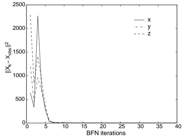
**Fig. 3.** Mean square difference between the observations and the BFN identified trajectory for the 3 variables versus the number of BFN iterations.
