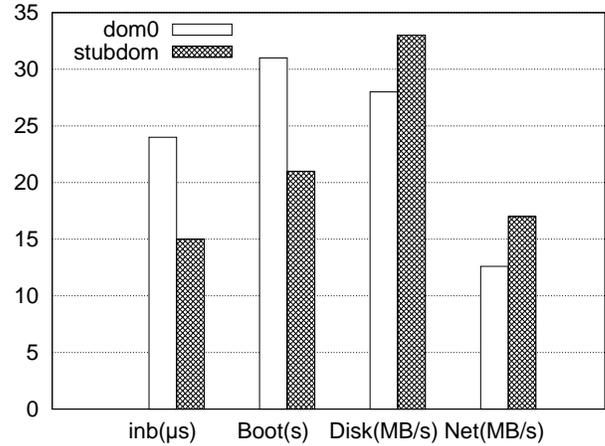
**Figure 5.** Performance of the fully virtualized guest, when *qemu* is running as a process in *dom0*, and when it is running in a *stub* domain: latency of guest I/O port access, guest boot time, throughput of disk and network.
