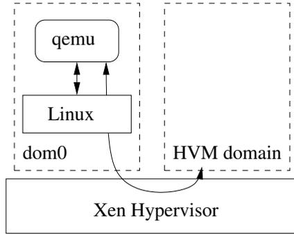
**Figure 3.** Traditional Xen approach: *qemu*, the device emulation component, runs as a process in *dom0*.
