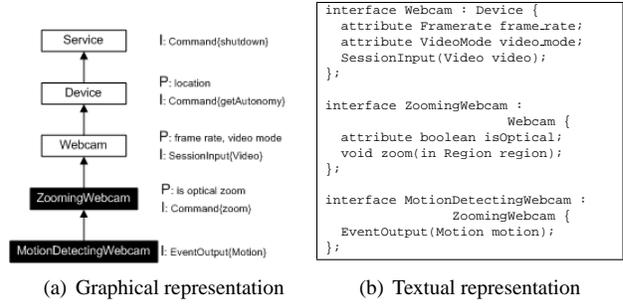
**Fig. 1. The zooming and motion detecting webcam**
