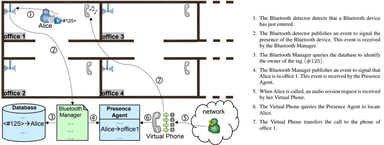
1. The Bluetooth detector detects that a Bluetooth device has just entered.
