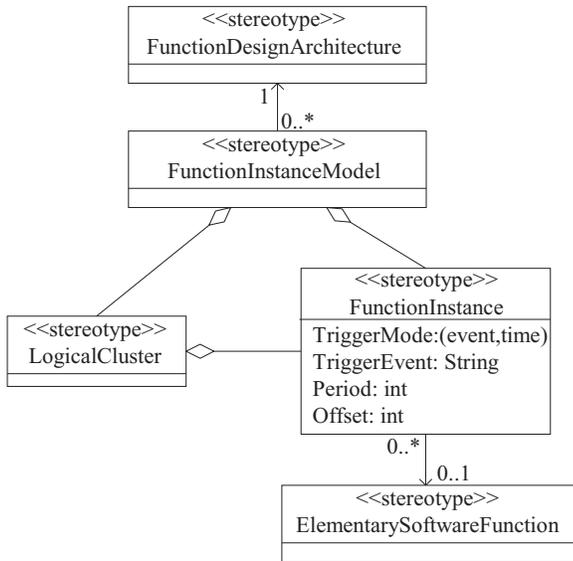
Figure 7. FunctionInstance specification
