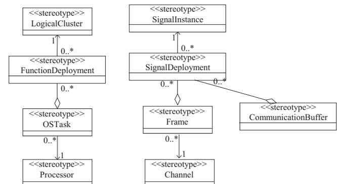
Figure 10. . Deployment model
