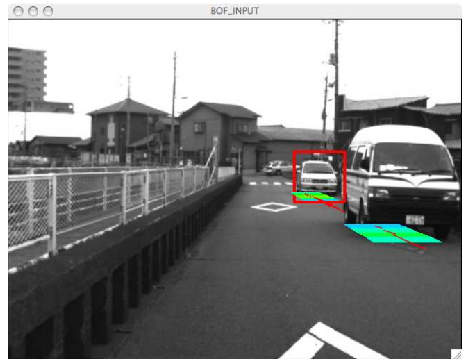
Fig. 1. Example of BOF output using a computer vision car detector as input (red boxes): The images are provided by a camera mounted on the moving ego-vehicle. The BOF output is projected back on the image. It represents a grid of occupancy probability (blue-to-red mapped color) and the mean velocity (red arrows) estimates.
