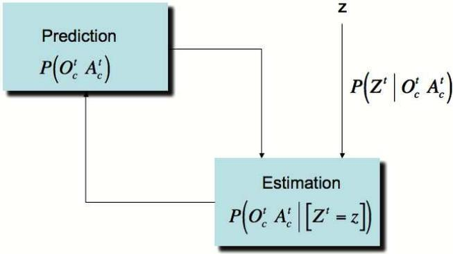
Fig. 4. Bayesian filtering in the estimation of occupancy and velocity distribution in the BOF grids
