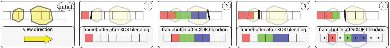
Figure 2: Solid Voxelization for a column in the slicemap. To simplify the illustration, only one framebuffer with two bit color channels is shown. Left: The scene, consisting of two watertight objects, is voxelized in the column along the view direction. 1-4): During rendering, fragments can arrive in an arbitrary order. For each fragment, a bitmask (upper row) is computed in the shader which indicates all voxels that lie in front of the current fragment. This mask is accumulated in the framebuffer (bottom, initialized at zero) using a XOR operation. Once the rendering is complete (4), the framebuffer contains a center sampled solid voxelization in a grid shifted by half a voxel.
