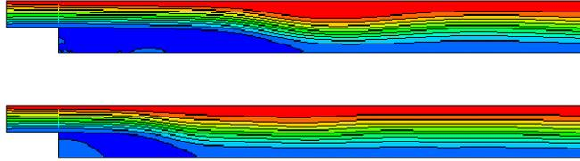
**Fig. 3.** Mean streamlines for uncontrolled (up) and non-intrusive *CLC* (down) regimes.
