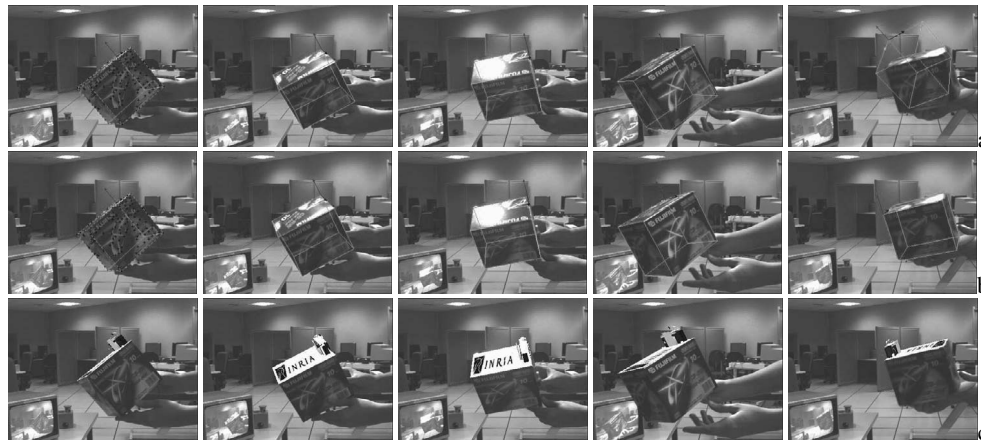
Figure 2. DVD box sequence. (a) tracking result using criterion \Delta_{2b} , (b) tracking result using criterion \Delta_{1b} . As one can see, though criterion \Delta_{2b} is supposed to better deal with specular changes, it fails sooner than the simpler criterion. (c) augmented image: the tracker is effective for such real-time applications.
