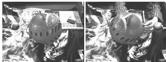
Figure 3. Ball sequence: augmented reality application. Even if the ball rotates around itself, which makes the specularities to occur step by step on the whole texture model, the tracker is effective for augmented reality applications.
