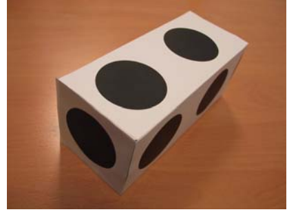
Fig. 2. 3D object employed in the camera calibration experiments.
