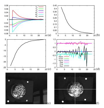
Fig. 2.  $1^{\text{st}}$  experiment (x axes in seconds).  ${}^d\Phi=0$ . (a) Kinematic screw (m/s or rad./s). (b) Error defined as  $\|\mathbf{e}\|$ . (c) Magnitude of the rotation  $\theta$  (deg.) (d) Vector  $\alpha$  in a fixed frame (filtered and non-filtered). (e) Initial image. (f) Final image.
