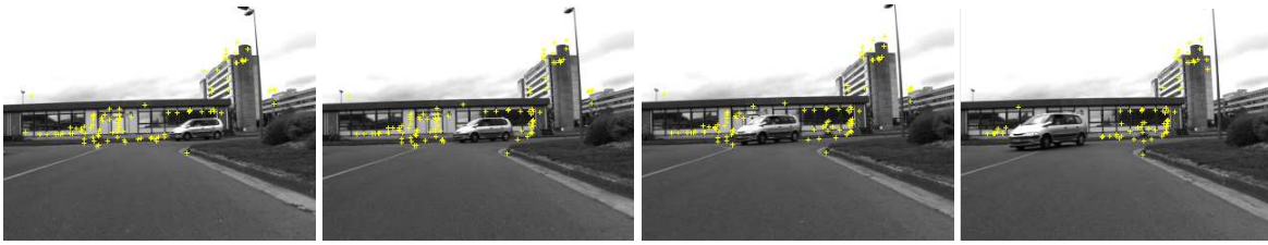
Fig. 6. Sequence from experiment 1 demonstrates robust feature (yellow crosses) tracking resumption after occlusion by a passing car.
