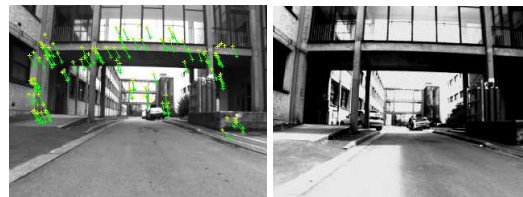
Fig. 8. Difference between the lighting conditions during navigation (left image) and mapping (right image) in experiment 2. Lines connect corresponding features in the current and reference image.
