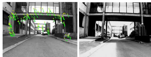
Fig. 8. Difference between the lighting conditions during navigation (left image) and mapping (right image) in experiment 2. Lines connect corresponding features in the current and reference image.
