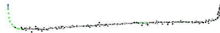
Fig. 7. Representation of the more than 240m reference path (green dots) using visual odometry for experiment 2. Robot locations during driving are shown as black dots.
