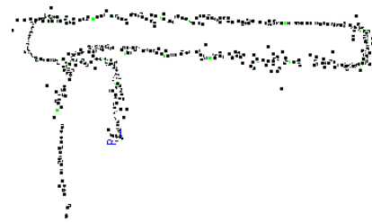
Fig. 12. Larger noise in the reconstructed robot poses where all features are far away in experiment 3.
