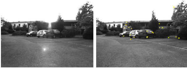
Fig. 15. Sun shining into the camera in the reference image (left) of exp. 4, but not in the current image (right) during navigation.
