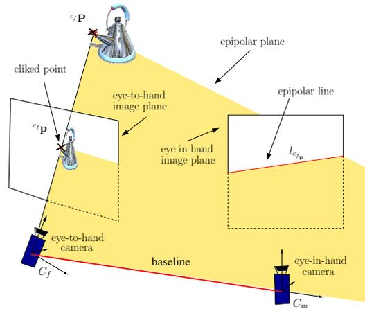
Fig. 5. Epipolar geometry of the eye-to-hand/eye-in-hand system
