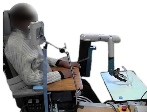
Fig. 3. The AVISO system consists of a MANUS arm [17], [33] mounted on a wheelchair, a stereo vision system fixed on the end effector of the arm, a graphical interface displayed on a monitor, any device adapted to the user's handicap (speech recognition, head movement, breath controller, joystick, etc. )
