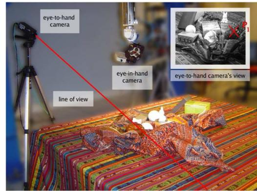
Fig. 7. Experimental setup: the scene is complex and the background is textured. The two camera locations are highlighted. Top right, the eye-To-Hand view is display with the clicked point  ${}^{cf}\mathbf{p}$ . The green line represents the line of view associated with  ${}^{cf}\mathbf{p}$
