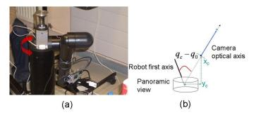
Fig. 2. Panoramic-based arm positioning: (a) the omnidirectional camera mounted onto the MANUS first axis, (b) the panoramic-embedded camera's relation when the second one is correctly aligned.
