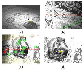
Fig. 6. Method illustration: (a) eye-to-hand view, with the user click (b) initial eye-in-hand view, with the current epipolar line in green and its desired position in red, (c) view during line scanning, (d) final FOV of the camera.
