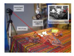
Fig. 5. Experimental setup, with a cluttered scene. The red line, defined by the user click, is the epipolar line that is covered by the embedded camera.
