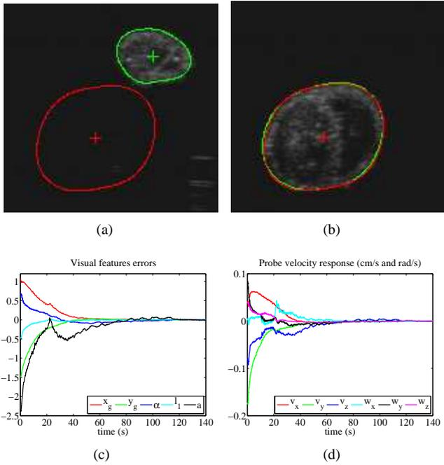
Fig. 8. Results from *in-vitro* experiment: (a) Initial (green) and desired (red) image sections edges before applying visual servoing - (b) Current (green) and desired (red) after applying visual servoing (c) Visual error response (cm, cm, rad, cm and  $\text{cm}^2$ ) - (d) Velocity applied to the probe
