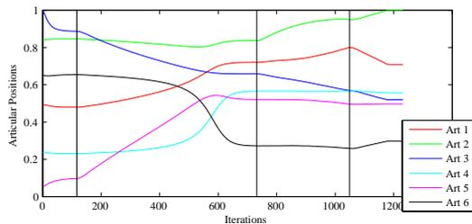
Fig. 4. Articular trajectories using the stack with the GPM but without stack controller. The limit is avoided during the execution of the third task ( $\mathbf{e}_z$ ) by moving along the axis 1. The robot reaches its joint limit during the last task, when no DOF are available any more.
