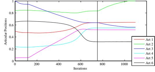
Fig. 3. Articular trajectories using the stack without any avoidance law. The second articulation (z-motion of the camera) reaches its limit during the execution of the third task (task  $e_z$ ). (each vertical line corresponds to the addition of a new task in the stack.)
