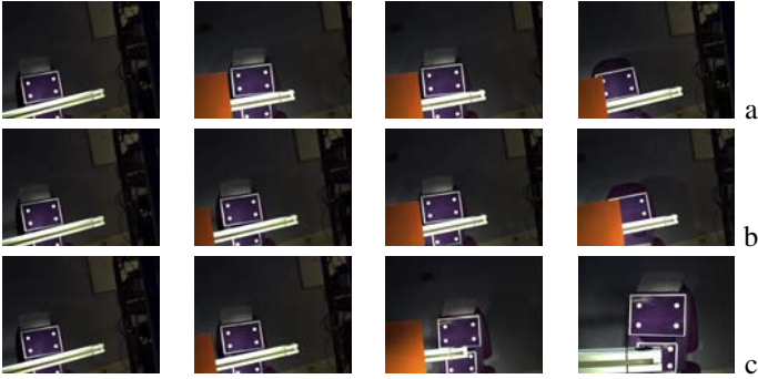
Fig. 7. Main phases of the servo without avoidance (a), with the avoidance law projected by the classical redundancy formalism (b) and with the control law projected by the proposed method (c). The pictures are taken by the embedded camera. The visual target is the four-white-points rectangle. The occluding object cared by a second robot is the orange shape that appears in the left of the image.
