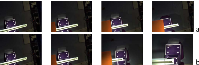
Fig. 6. Main phases of the servo with the avoidance law projected using the classical redundancy formalism (a) and using the proposed method (b). The pictures are taken by the embedded camera. The visual target is the four-white-points rectangle. The occluding object carried by a second robot is the orange shape that appears in the left of the image.
