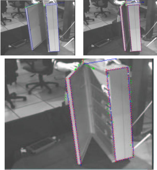
**Figure 4.** Rotation of a hinged door whilst undergoing movement. In this and all the following figures the reference frames for each component are shown as well as a projection of the CAD model onto the image. The axes of the frames are drawn in yellow, blue and red. The contour of the object is shown in blue. The points rejected by the M-estimator are shown in green.
