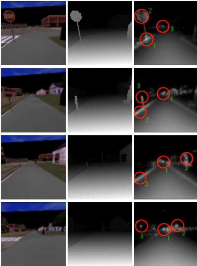
**Fig. 4.** Different saliency maps obtained during the wandering. First column shows the corresponding subjective view, second column shows the depth buffer and the last column is the saliency map with the location of three fixations
