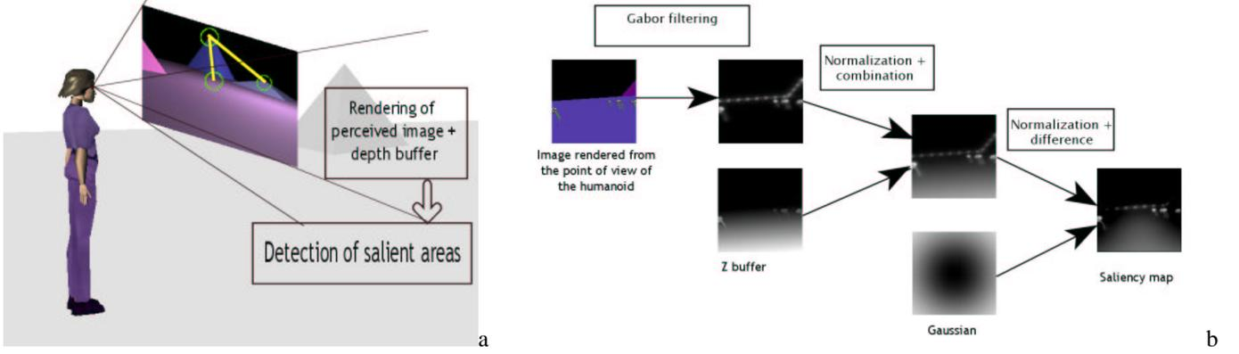
**Fig. 1.** (a) Using saliency map to perceive the environment. Green circles are conspicuous zones, and the yellow lines are a pathway between those zones (b) obtaining a saliency map based on spatial frequencies and depth information
