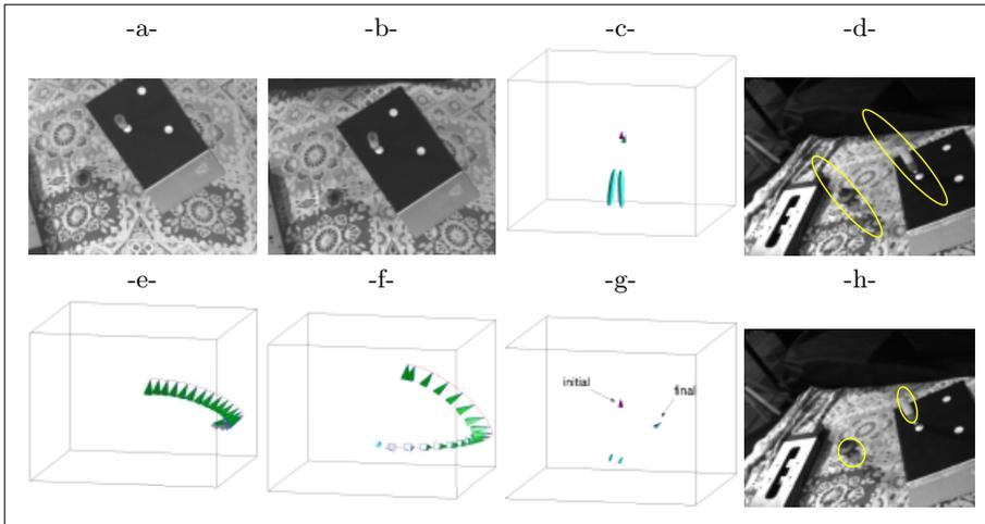
**Fig. 5.** Two objects reconstruction. a,b-Initial images. c- First estimation of the including ellipsoids. d- Associated projection in the last image. e- Locally optimal exploration. f- Best view point exploration. g- Final reconstruction for the best view point strategy. h- Associated projection in the final image.
