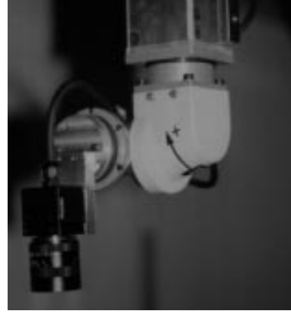
Fig. 7. Camera mounted on the end-effector of an Afma cartesian robot.
