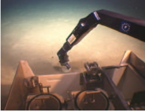
Figure 2: The Victor 6000 six dof manipulator Maestro (© Ifremer)
