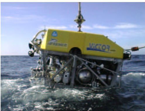
Figure 1: The Ifremer Victor 6000 underwater ROV (© Ifremer)
