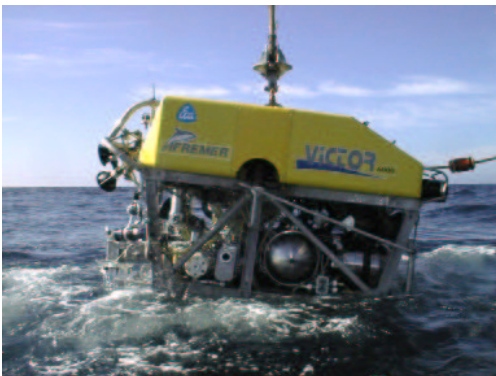
Figure 1: The Ifremer Victor 6000 underwater ROV (© Ifremer)
