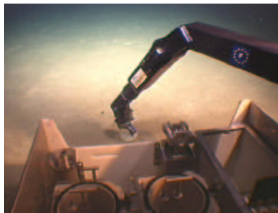
Fig. 2. The Victor 6000 six dof manipulator Maestro (© Ifremer)
