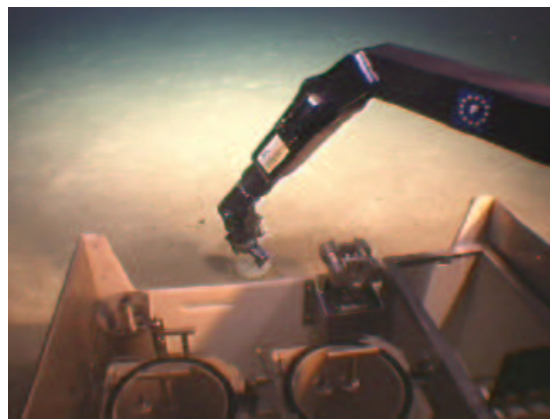
Fig. 2. The Victor 6000 six dof manipulator Maestro (© Ifremer)
