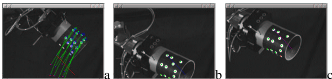
Fig. 5. Effect of the pan/tilt control: the desired position of the object in the image is modified. (a) initial position, (b) desired position with no pan/tilt control, (c) desired position with pan/tilt control.
