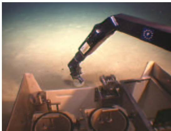
Fig. 2. The Victor 6000 six dof manipulator Maestro (© Ifremer)
