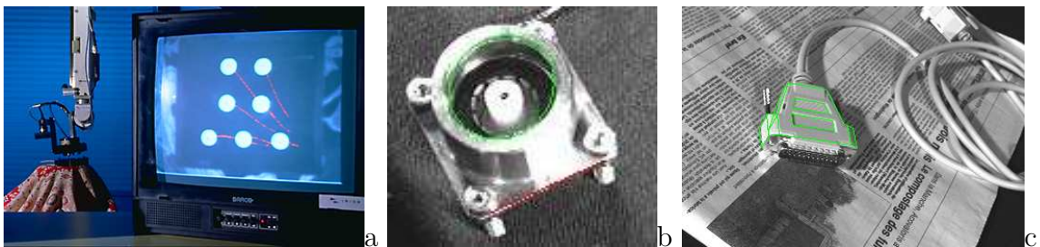
Figure 1: Tracking features for visual servoing robotic tasks: three levels of complexity (a) tracking artificial landmarks (white dots) for a grasping task (b) tracking specific geometrical features (ellipse and segment) (c) tracking complex objects (a connector) in a textured environment.
