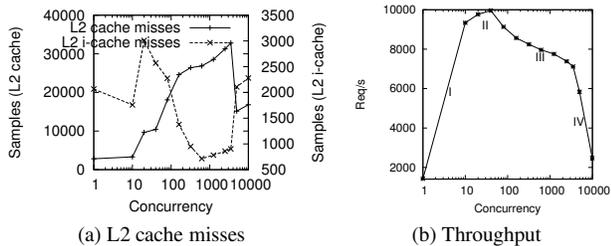
**Figure 3.** Throughput degradation with increasing L2 cache misses.
