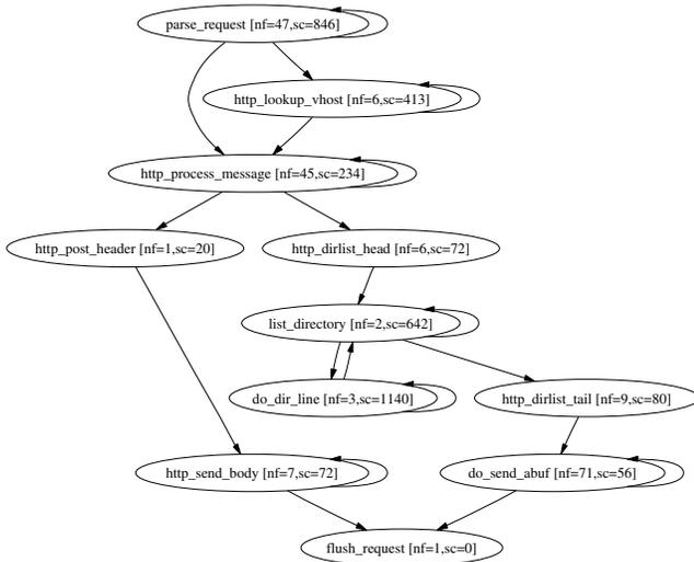
**Figure 7.** A fragment of the Stage Call Graph (SCG) of TUX.  $nf$  denotes the number of functions in a stage, and  $sc$  its maximum stack utilization in bytes. Functions belonging to the same stage have been collapsed into a node representing the stage.
