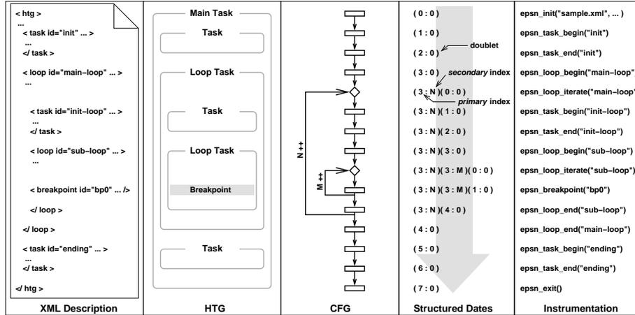
Fig. 4. Comparison of the different representation modes.
