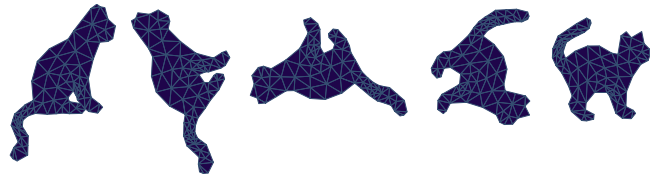
Figure 8: Minimizing rotation: Results like the above can arise from naïve application of the rotation consistency fix. The entire cat rotates around its tail because of an unlucky choice of initial triangle. Compare with corrected minimal rotation sequence in Figs. 5 and 6.
