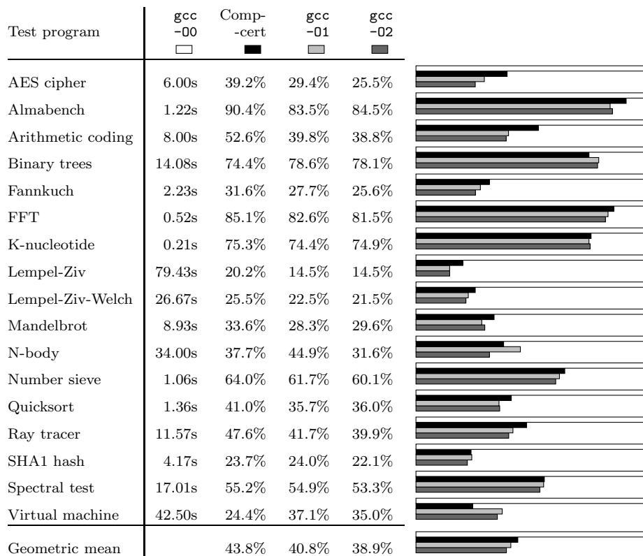
Fig. 19 Execution times of compiled code. Times are given relative to those obtained with gcc -00. Lower percentages and shorter bars mean faster.
