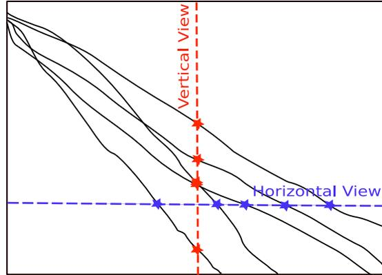
Figure 4: Illustration of vertical-cut and horizontal-cut view. Black lines depict the best function value plotted versus number of function evaluations.
