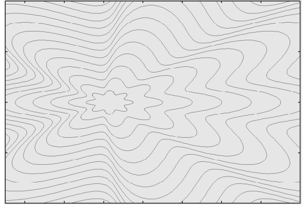
Figure 7: Here, the t level set is \{\frac{1}{10}t + t \times (1 + 0.2 * \cos(8u)) \times \cos(u), t \times (1 + 0.2 * \cos(8u)) \sin(u); u \in [0, 2\pi]\} . Due to dissymmetry, the center of the level set if not the optimum and the condition of the theorem are not met. However, it is clear that the algorithm will converge in this case as well as we don't have to be exactly centered on the optimum. This will be discussed on a similar problem in section 5, see in particular Fig. 11.
