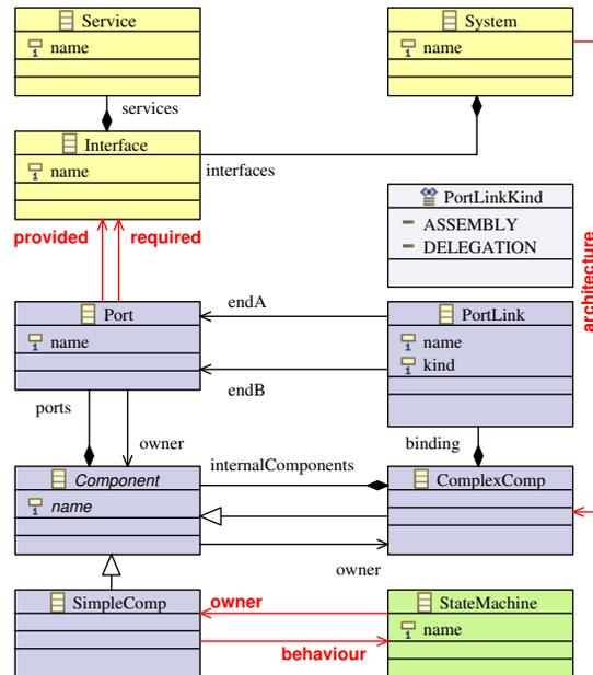
**Figure 1. The V<sup>3</sup>Studio structural view (component diagrams). The red association links define the relationships between the architectural and behavioral views and between the definition of components and interfaces. These associations make it possible to reuse previously defined models.**
