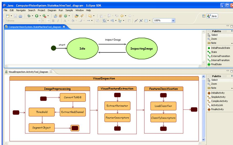
Figure 5. Models developed as part of the vision-guided robotic system case study. *Top*: Computer\_Vision\_System coordination view, *Bottom*: Activity diagram associated to the InspectingImage state.
