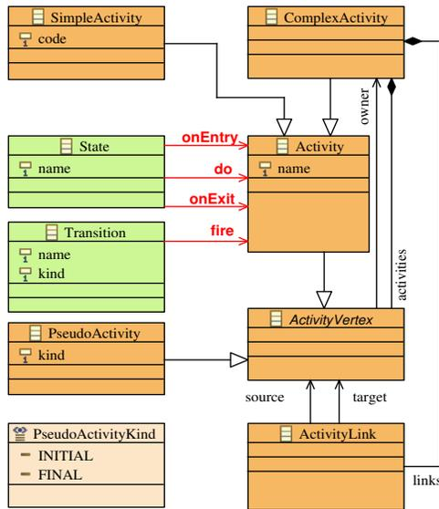
**Figure 3. The V<sup>3</sup>Studio algorithmic view (activity diagrams).**
