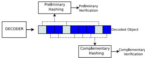
Fig. 2. VeriFEC preliminary versus complementary integrity verification.
