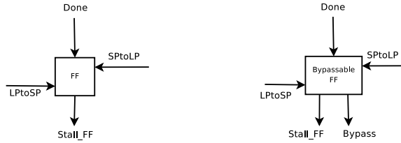
Figure 10: Centralized implementation building blocks.
