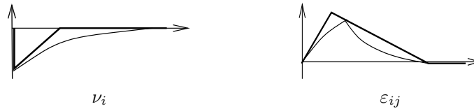
Figure 3: Potential profiles used in equation (12). The original exponential profiles derived by the authors of the model are shown as thin curves and the piece-wise linear approximation as thick lines. Any other piece-wise linear profiles could be considered, including piece-wise finer linear approximation of exponential profiles.
