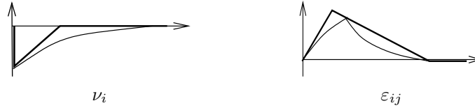
Figure 3: Potential profiles used in equation (12). The original exponential profiles derived by the authors of the model are shown as thin curves and the piece-wise linear approximation as thick lines. Any other piece-wise linear profiles could be considered, including piece-wise finer linear approximation of exponential profiles.
