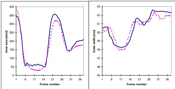
Figure 4. Left : Inner contour area ( $\text{mm}^2$ ); Right : Outer contour width (mm); measured parameter is in dot line, predicted in full line.
