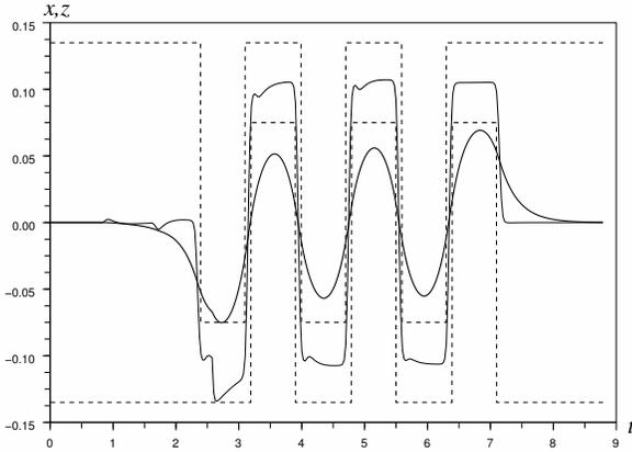
Fig. 6. Online recomputation of the trajectory of the Center of Mass of the robot with the ZMP Preview Control scheme, taking into account the perturbation at time  $t = 2.5$  s generated by a mass corresponding to 20% of the total mass of the robot. Note that the limits on the position of the CoP that appear here and in the following figures lie 4 cm inside the feet for safety reasons.
