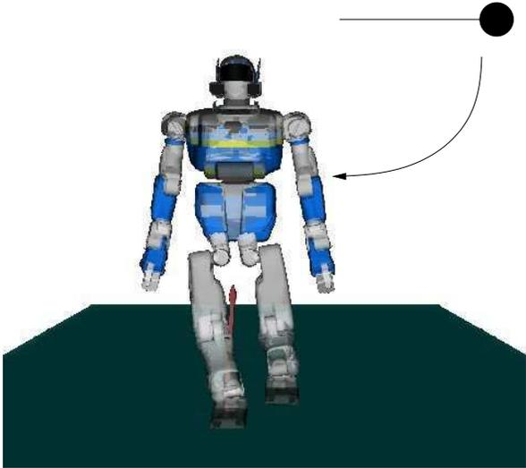
Fig. 4. The perturbation considered here corresponds to a mass  $M$  hitting the robot in the middle of the trunk from the side after having fallen from a height of  $0.5\text{ m}$  under the action of gravity.
