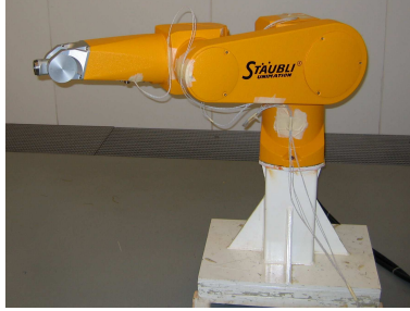
Figure 7: Flat configuration of a Staubli Rx90
