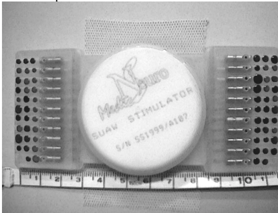
Fig. 1 The implant with its ceramic box where the electronic is encapsulated, and the connectors : 2 common anodes and 12 cathodes for epimysial stimulation, 4 anodes and 4 cathodes for neural stimulation.
