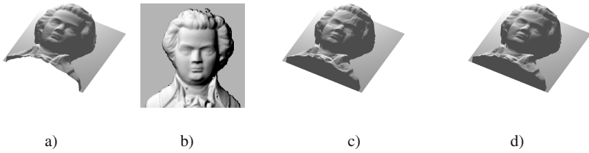
Fig. 1. a) original surface (groundtruth); b) image synthesized from a); c) surface reconstructed by using the classical causality; d) surface reconstructed by our algorithm
