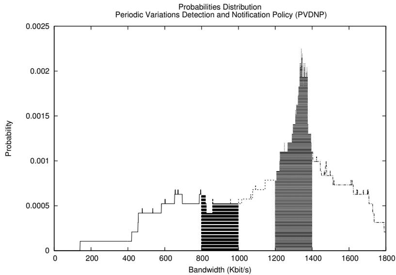
**Figure 12.** Probabilities distribution of the bandwidth when the periodic algorithm is used
