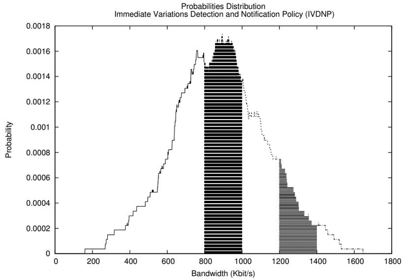
**Figure 11.** Probabilities distribution of the bandwidth when the immediate algorithm is used
