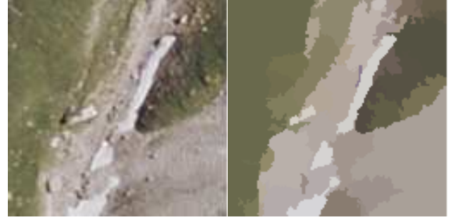
Figure 3: A sample of high resolution aerial image [14] (left) and its corresponding unsupervised segmentation (right)
