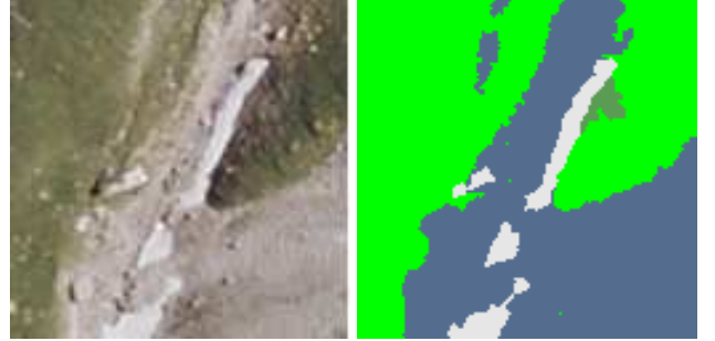
Figure 6: Image classification correction. Original aerial image (left), class map (right)
