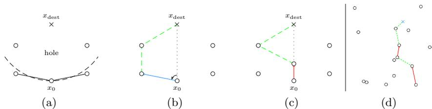
**Fig. 1.** Illustration of a *routing hole* in a WSN. (a) Node  $x_0$  is closer to the destination  $x_{dest}$  than its neighbors making greedy routing fail. (b) Face-based routing algorithms route along the edges bordering the void while (c) Grasp leverages the node mobility to move toward the destination until greedy forwarding is possible. (d) Sample path using GRASP. Dashed lines denote *greedy forwarding* and solid lines and arrows denote respectively hole circumventing and moving.
