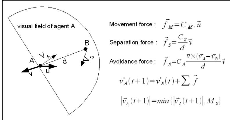
**Fig. 4: Forces in the pedestrians system.** Computing of the new speed of an agent A, that has a single agent B in its visual field. We assimilate the sum of forces to the acceleration because the mass of the agent can be considered in the coefficients  $C_m$ ,  $C_s$  and  $C_a$  without adding a new parameter.
