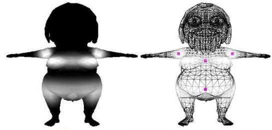
Figure 12: The breast, arms, belly and bottom of this Eva model have been animated in real-time using 4 connected flesh elements. The first image shows the dynamic skinning weights values at rest and the second image shows the positions of the local frames.
