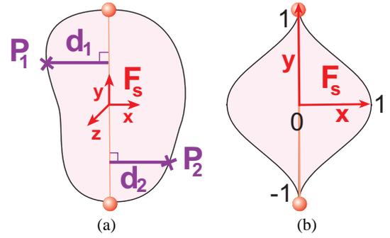
Figure 5: (a) : the weight given by the first constraint corresponds to the Euclidean distance between the vertex and the flesh element virtual bone. It corresponds to  $d_1$  for  $P_1$  and to  $d_2$  for  $P_2$ . (b) : the attenuation function that attenuates the weights given by (a).
