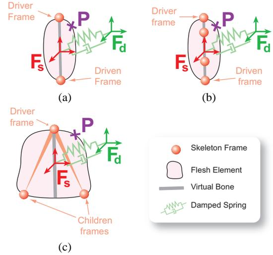
Figure 4: A dynamic frame  $F_d$  is connected to a local frame  $F_s$  through a damped spring of zero rest length. (a) and (b) : the local frame stands in the middle of the virtual bone delimited by two end joints. (c) : the local frame is defined by three end joints.
