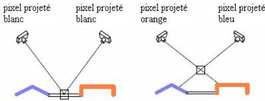
FIG. 3 – Principe de la photo-consistance [8]
