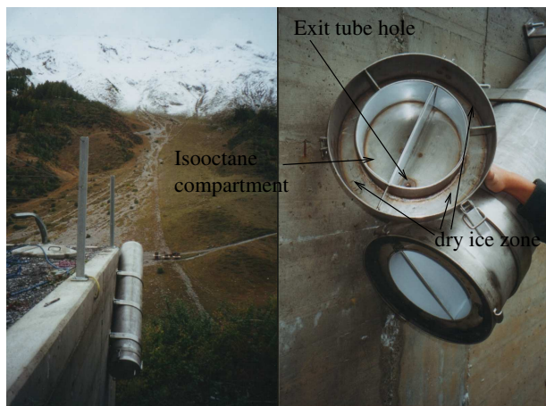
Figure 3: Left: the experimental device fixed on the bunker of the experimental test site of vallée de la Sionne (Switzerland). Right: the removable bottom.
