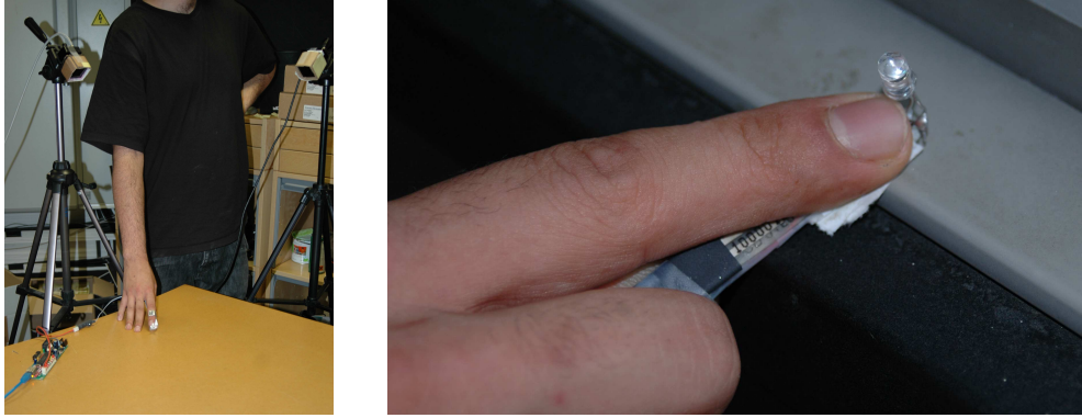
Figure 3: Opportunistic music prototype. (left) General setup with camera pair, finger mounted FSR+LED interaction device, FSR analog acquisition board. (right) Close-up of the thimble interaction device, with FSR sensor and infrared LED.
